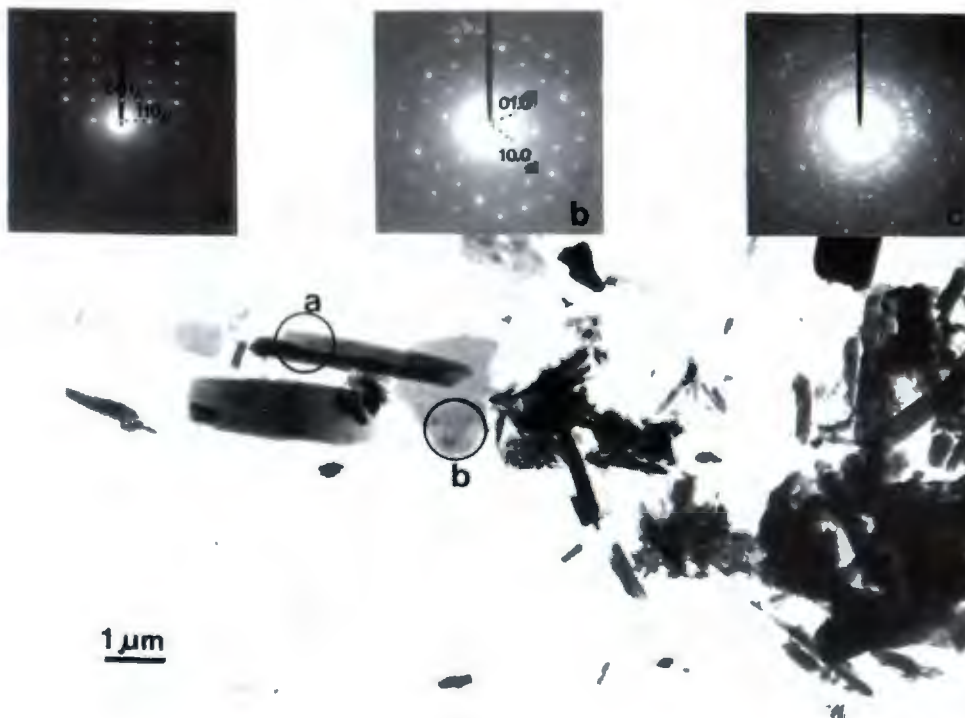
Fig. 3 TEM micrograph of recent surface sediment from Malo Jezero, with diffraction patterns of (a) needle-like particles of aragonite, (b) plate-like grains of calcite, and (c) polycrystalline ring pattern taken from a cluster.
