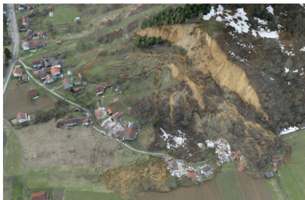
Fig. 1.3. 3D model of the landslide “Kubarnovo brdo – Stari put”, based on aerial photos (drone data) showing clear landslide features (Croatian Geological Survey, March 14 th 2018) (PODOLSZKI et al., 2018a).
