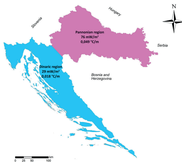
Fig. 2.1. Schematic division of the Croatian territory according to geothermal features (modified from BOŠNJAK et al., 1998).
