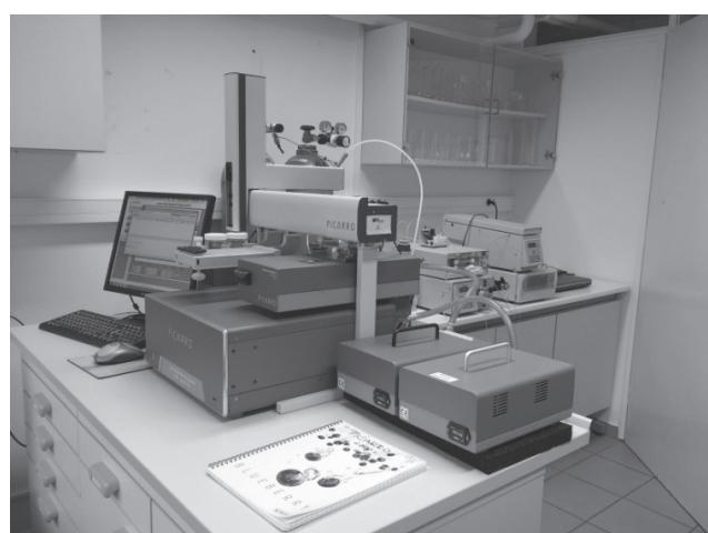
**Figure 1.** The Picarro L2130i instrument.
